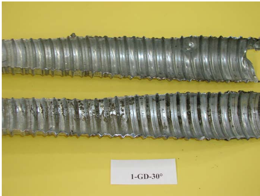
Figure 4-21 Damage in specimen 1-GD-30°
