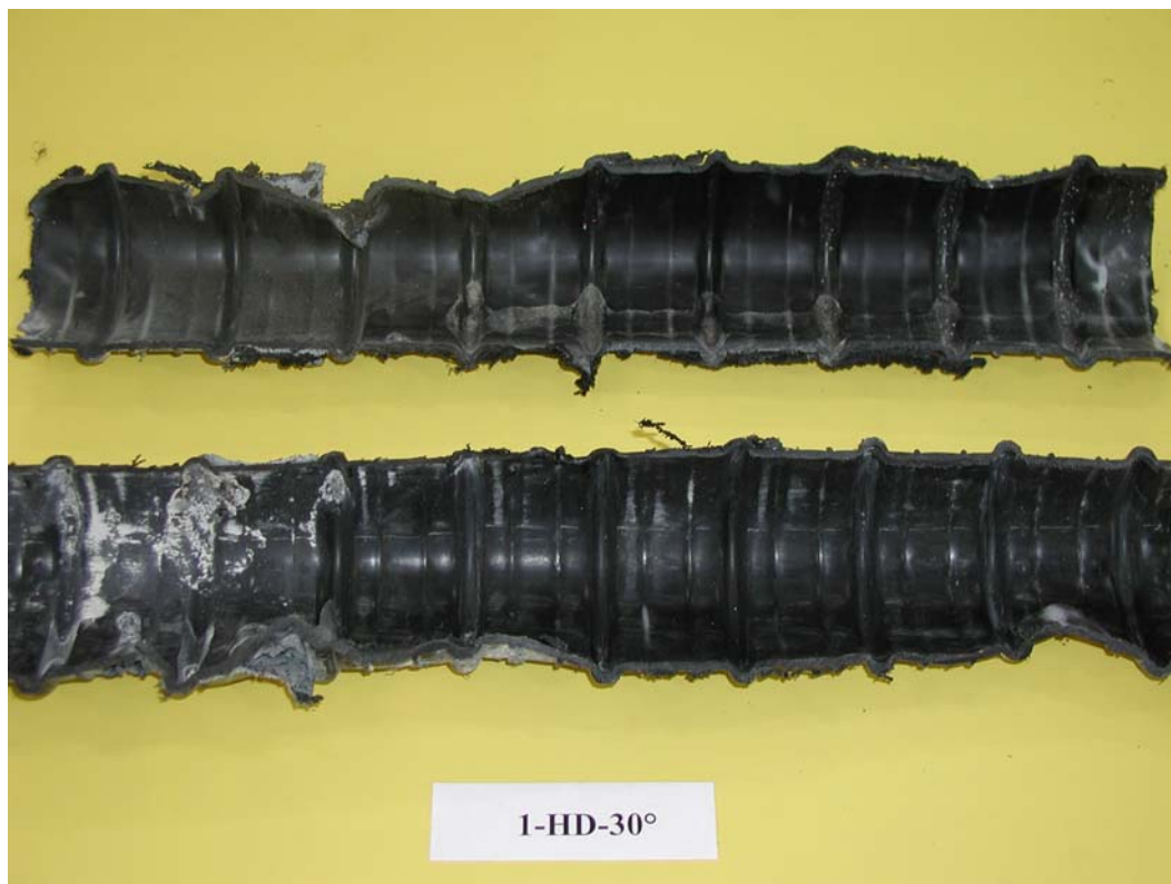
Figure 4-17 Damage in specimen 1-HD-30°
