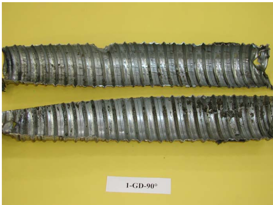
Figure 4-22 Damage in specimen 1-GD-90°
