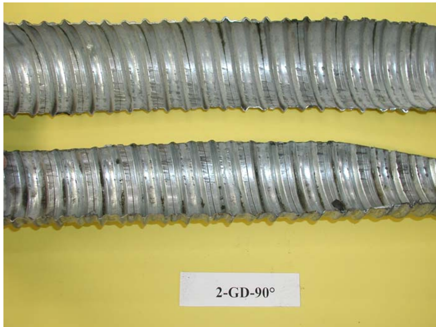
Figure 4-24 Damage in specimen 2-GD-90°
