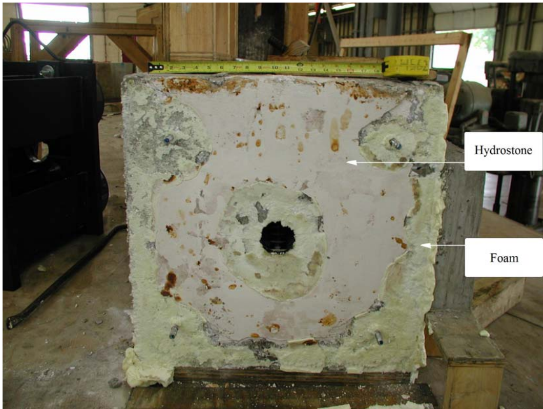
Figure 3-15 Hydro-stone on face of beam
