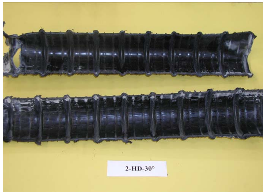
Figure 4-18 Damage in specimen 2-HD-30°
